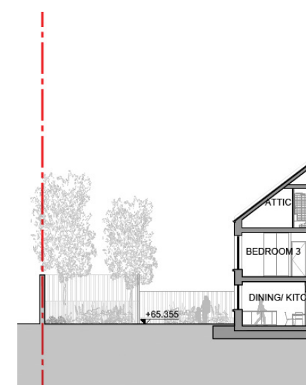
Site Section A-A - Boundary treatment (Refer to Drawing 2/301 Site Section A-A as part of this submission) **nts
